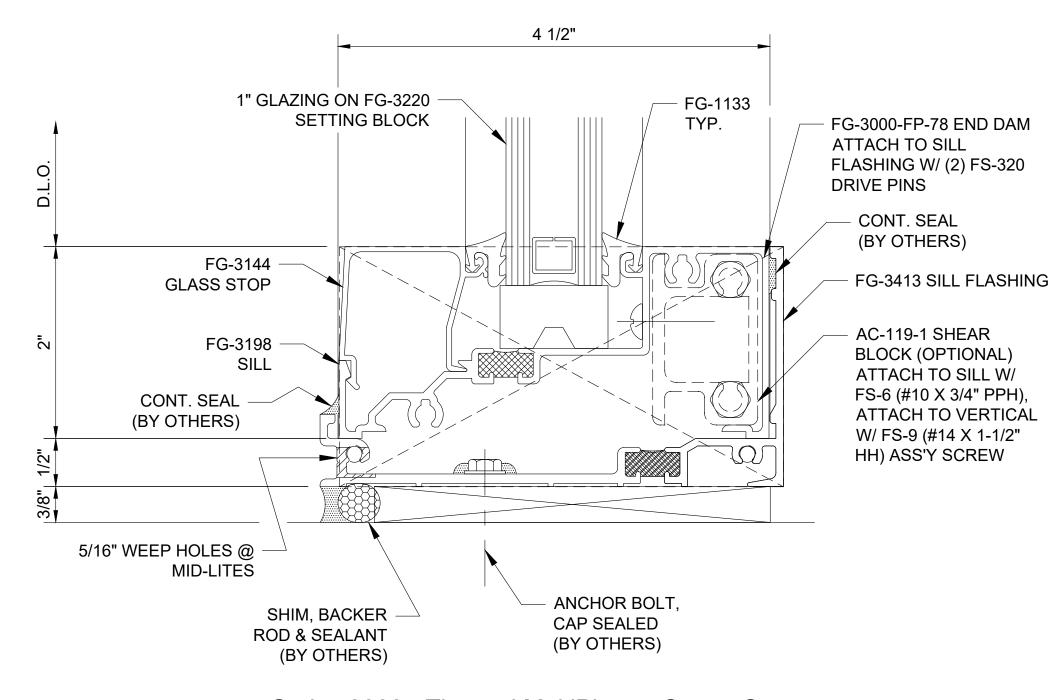
Series 3000 - Thermal MultiPlane - Center Set Sill Horizontal - H0910
