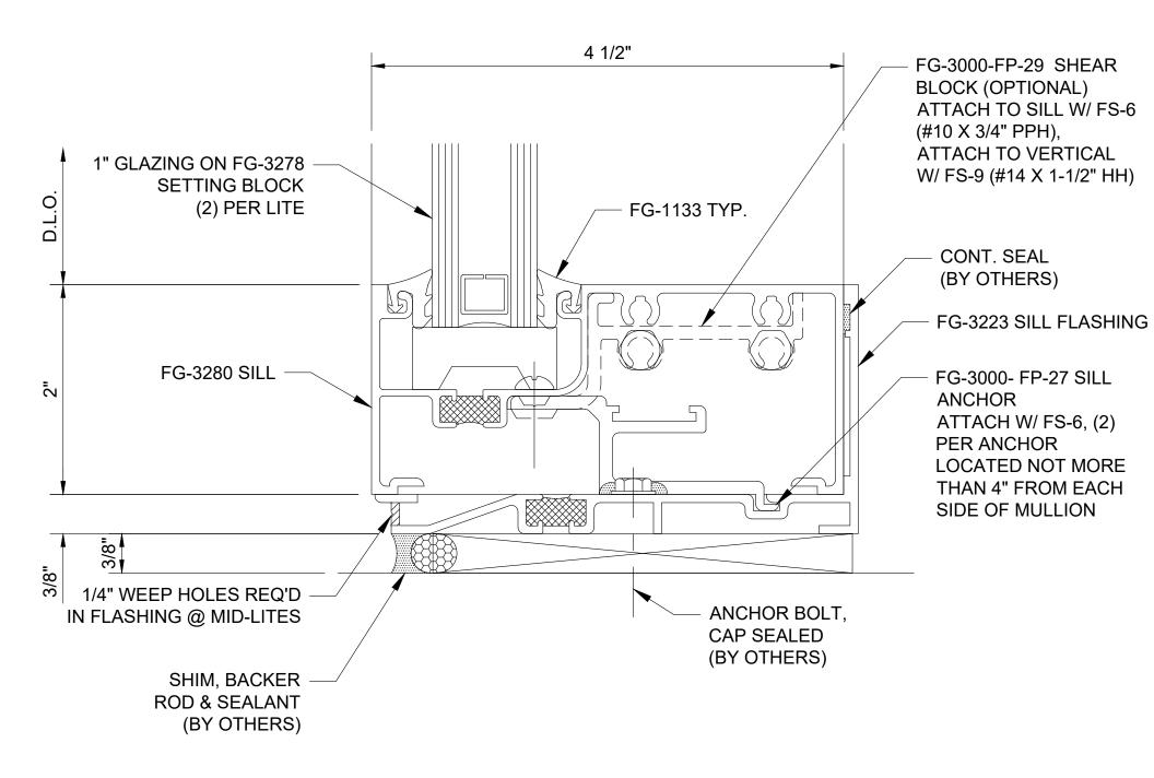
Series 3000 - Thermal MultiPlane - Front Set Sill Horizontal - H4109
