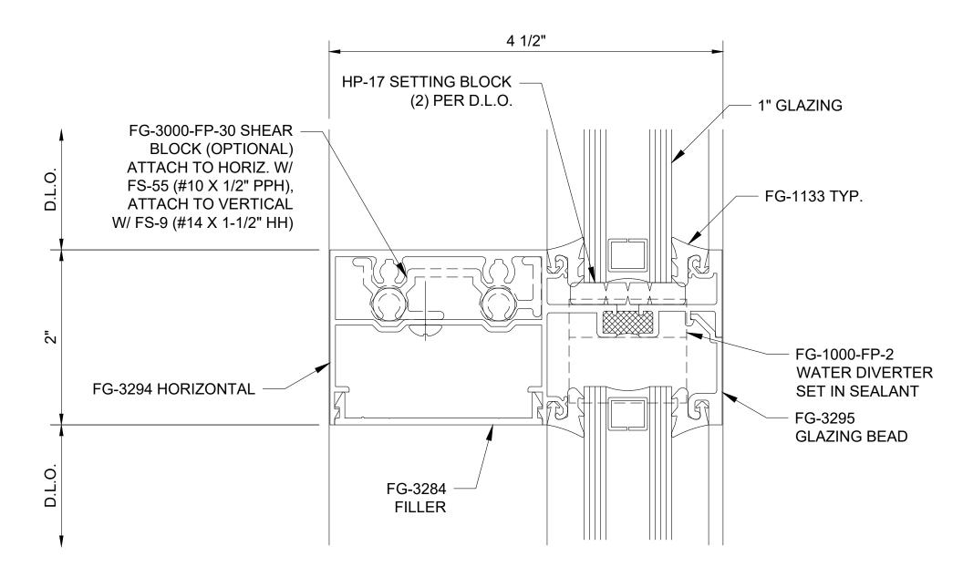
Series 3000 - Thermal MultiPlane - Back Set Intermediate Horizontal - H4514
