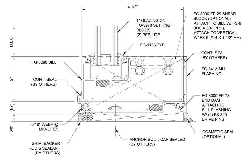
Series 3000 - Thermal MultiPlane - Front Set Sill Horizontal - H4103
