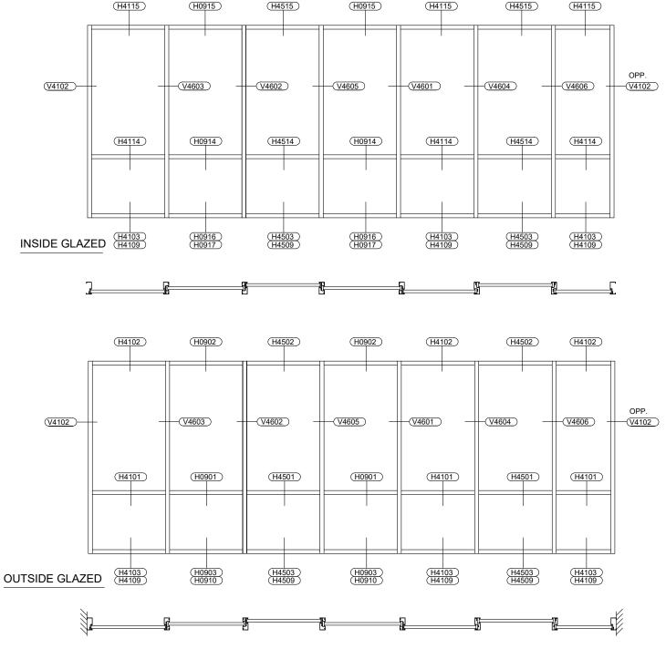
Series 3000 Thermal MultiPlane Storefront - Multi-Set 2" x 4-1/2" w/ 1" Glazing - Elevation
