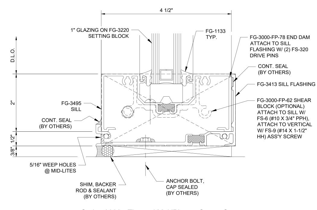
Series 3000 - Thermal MultiPlane - Center Set Sill Horizontal - H0917
