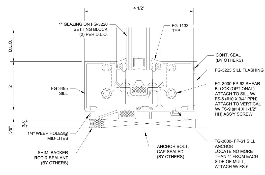
Series 3000 - Thermal MultiPlane Sill Horizontal - H0916
