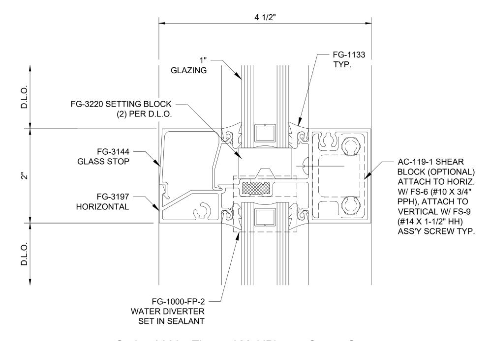
Series 3000 - Thermal MultiPlane - Center Set Intermediate Horizontal - H0901
