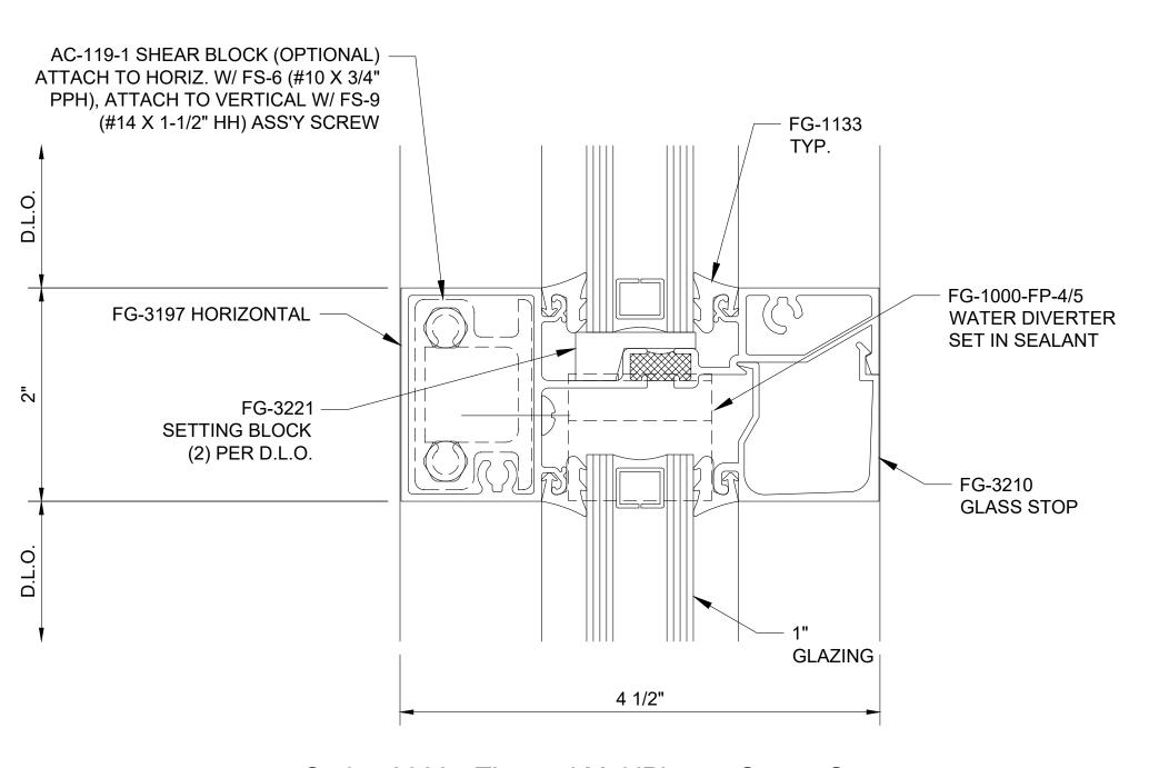
Series 3000 - Thermal MultiPlane - Center Set Intermediate Horizontal - H0914
