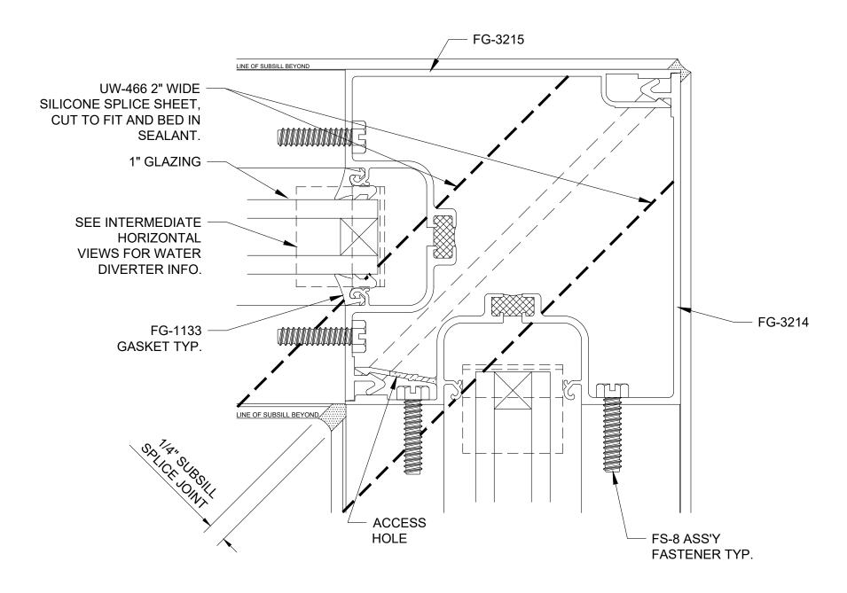
Series 3000 Thermal MultiPlane - Center Set 90° Inside Corner - V0912
