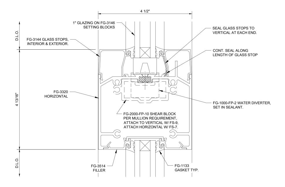
Series 3000 Thermal MultiPlane - Center Set Sidelite Base Horizontal - H0941
