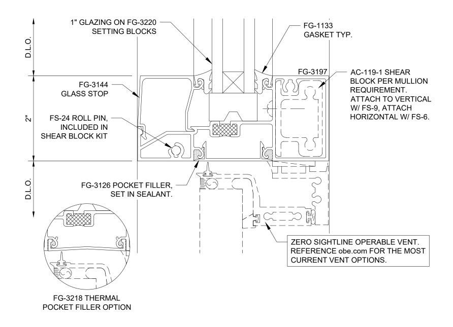
Series 3000 Thermal MultiPlane - Center Set Horizontal at Operable WIndow - H0919
