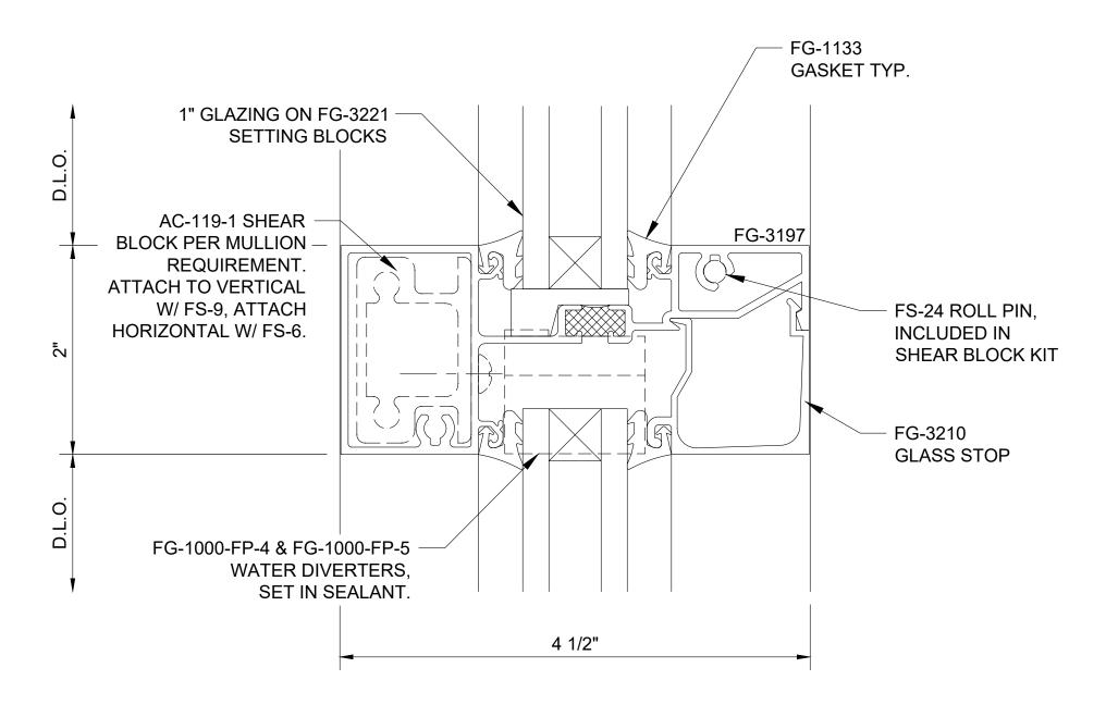
Series 3000 Thermal MultiPlane - Center Set Intermediate Horizontal - Inside Glazed - H0914
