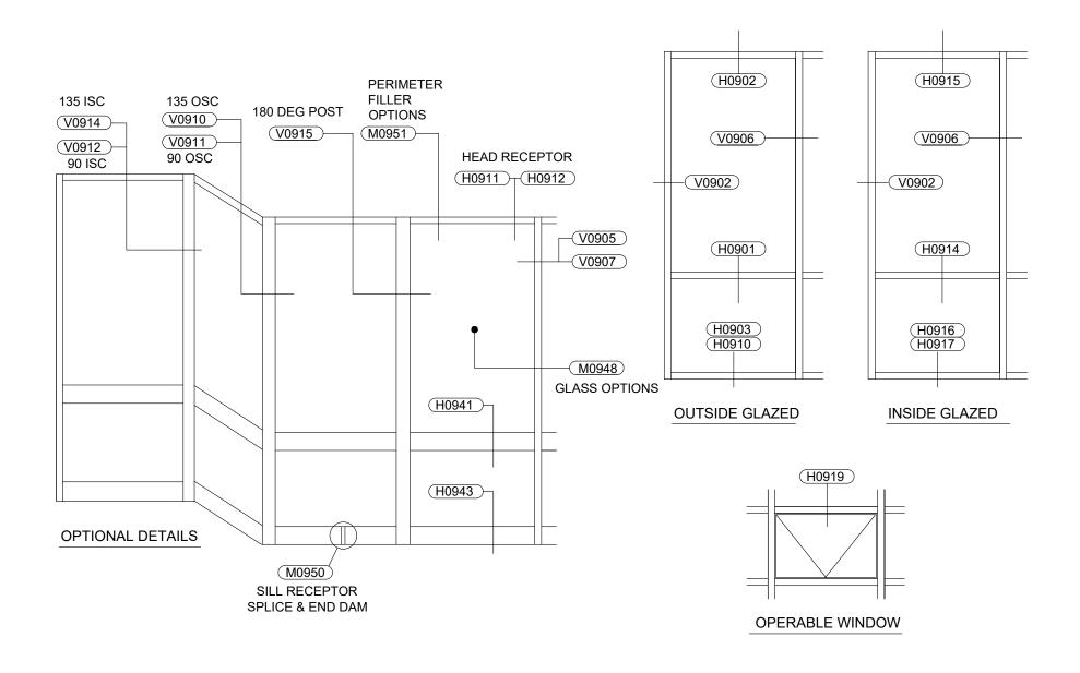
Series 3000 Thermal MultiPlane - Center Set 2" x 4-1/2" Thermally Broken Storefront for 1" Typ. Infill - Elevation
