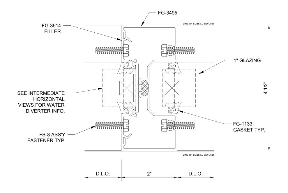
Series 3000 Thermal MultiPlane - Center Set Typical Vertical - V0906
