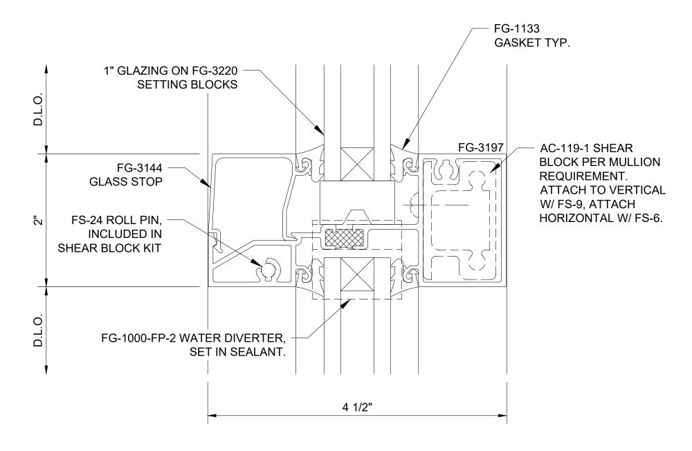
Series 3000 Thermal MultiPlane - Center Set Intermediate Horizontal - Outside Glazed - H0901
