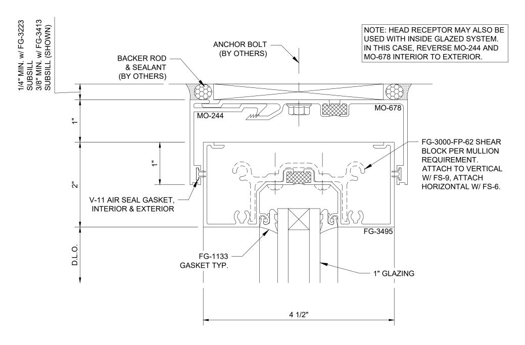
Series 3000 Thermal MultiPlane - Center Set Head w/ Receptor - H0912
