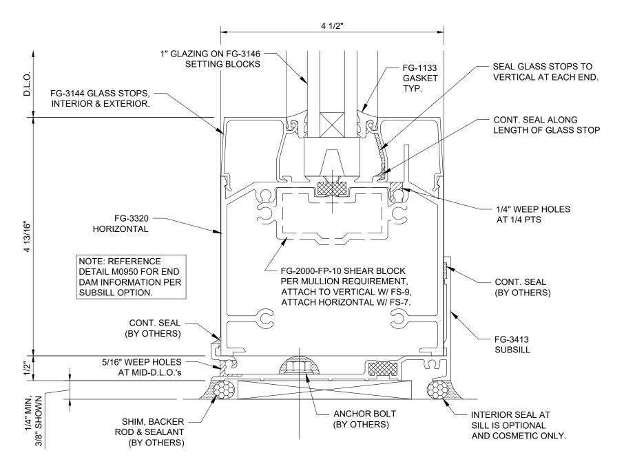
Series 3000 Thermal MultiPlane - Center Set Sidelite Base Sill - H0943
