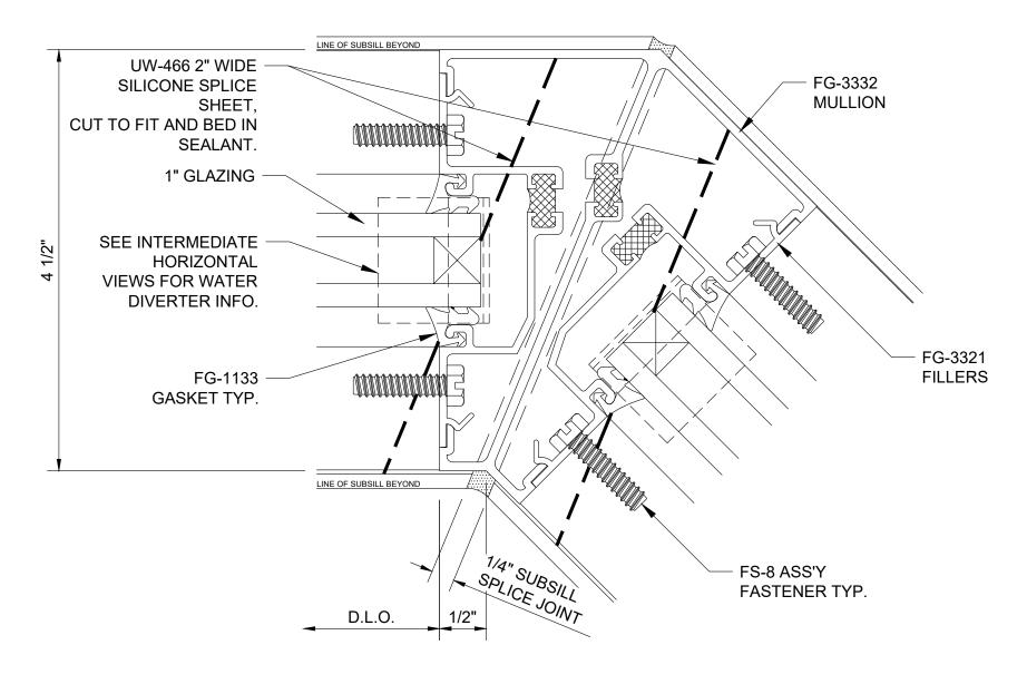
Series 3000 Thermal MultiPlane - Center Set 135° Inside Corner - V0914
