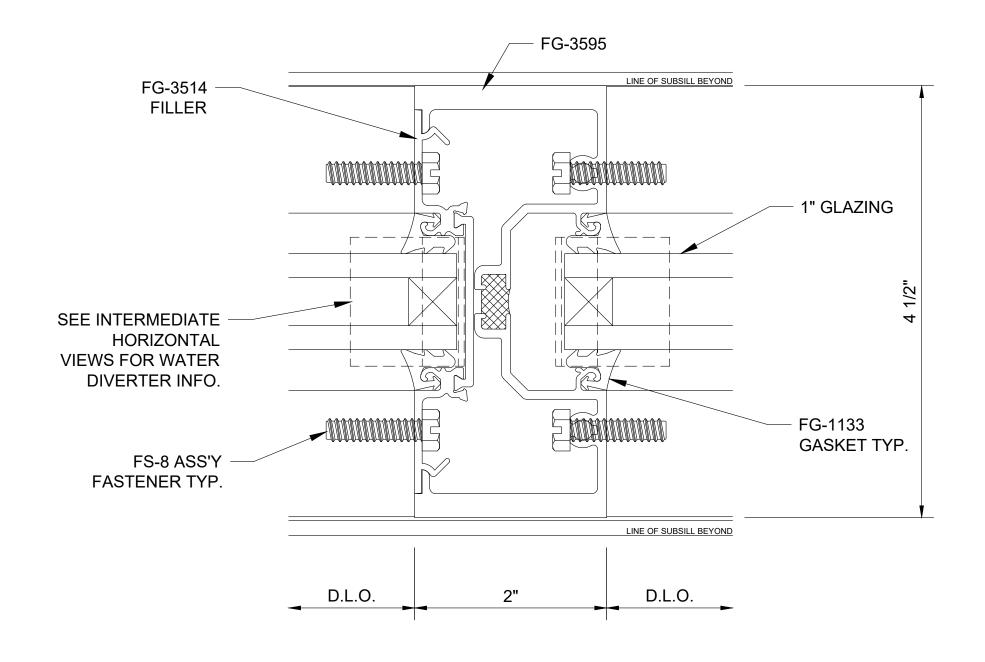
Series 3000 Thermal MultiPlane - Center Set Heavy Vertical - V0905
