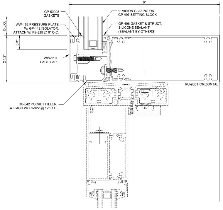
Reliance™ Unit Wall - Captured SSG Horizontal @ Thermal Door Header - H1882
