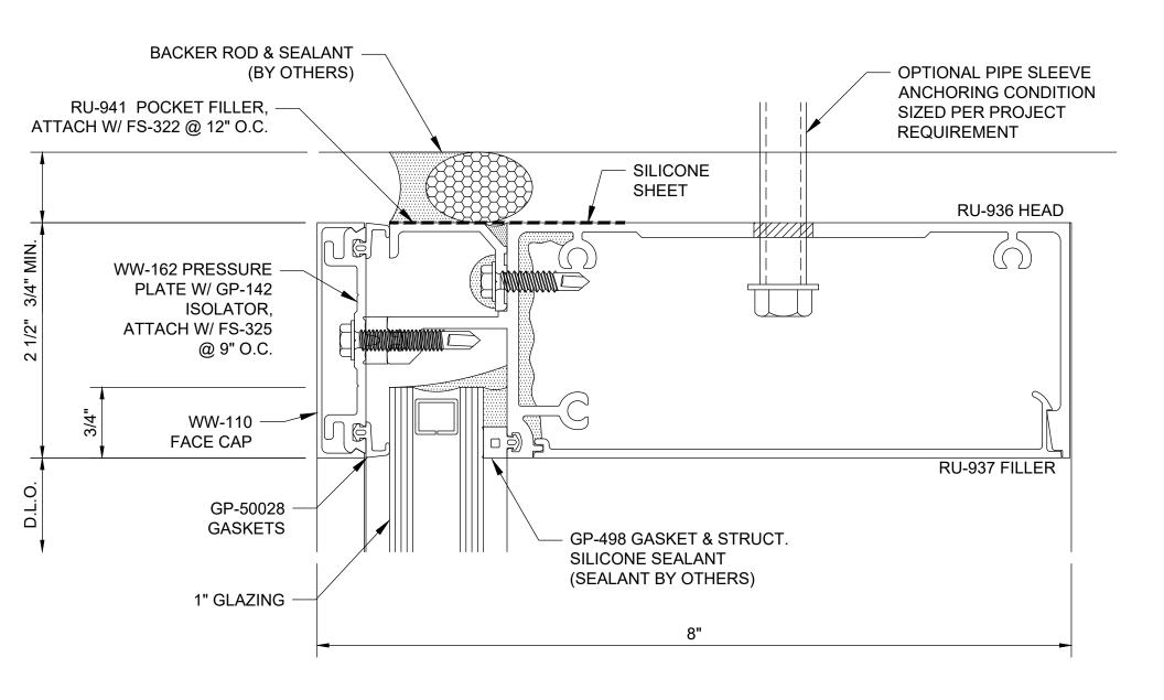
Reliance™ Unit Wall - Captured SSG Head Horizontal - Single Span - H1854
