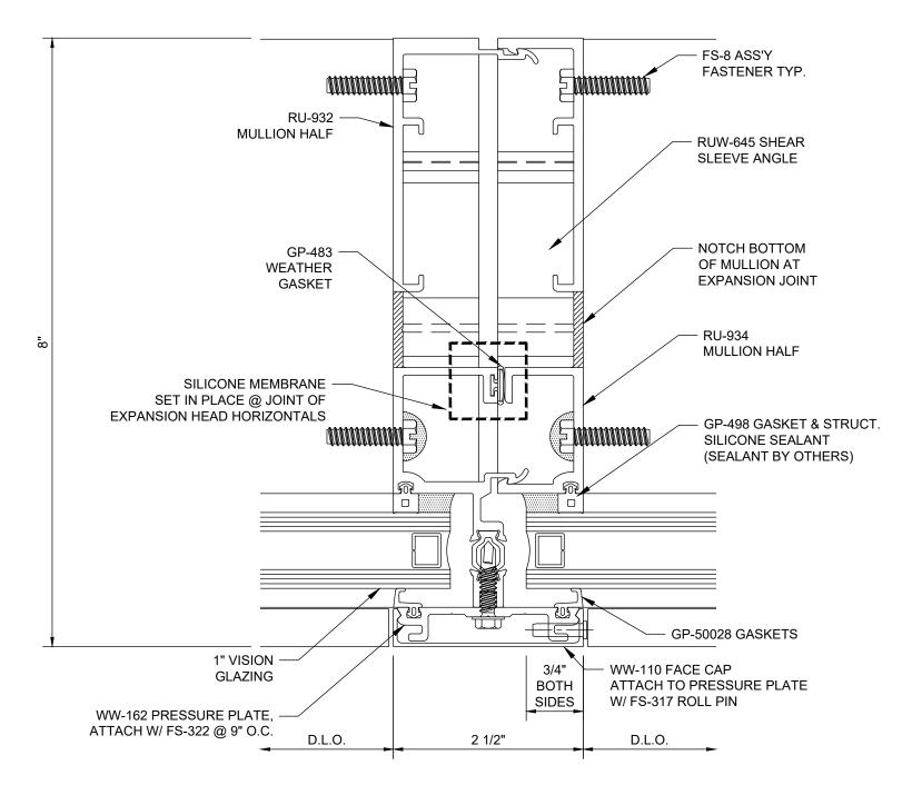
Reliance™ Unit Wall - Captured SSG Intermediate Vertical @ Stack Joint w/ Shear Sleeve Angle - V1864
