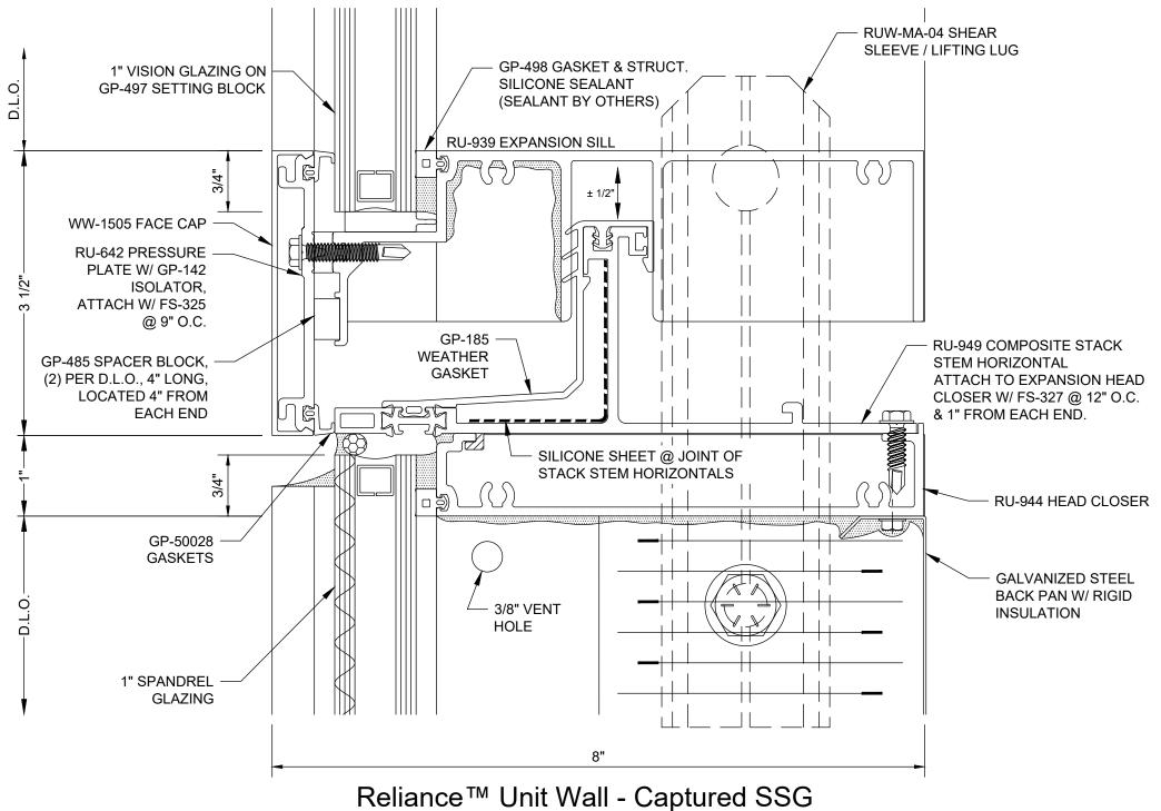
Stack Joint - Vision over Spandrel w/ Shear Sleeve/Lifting Lug - H1860
