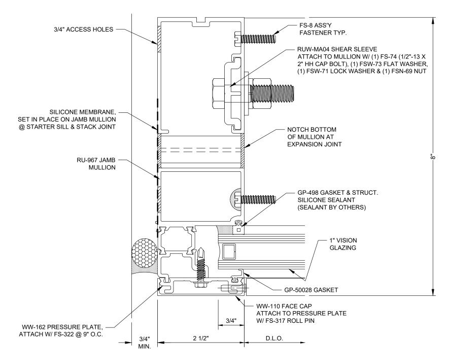
Reliance™ Unit Wall - Captured SSG Jamb Vertical @ Stack Joint - V1868
