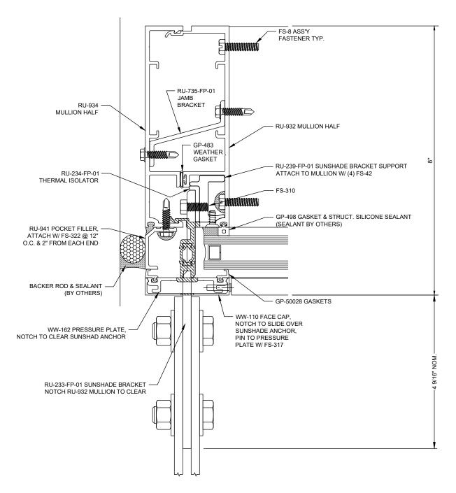
Reliance™ Unit Wall - Captured SSG Sunshade Anchoring at Jamb Vertical - V1890
