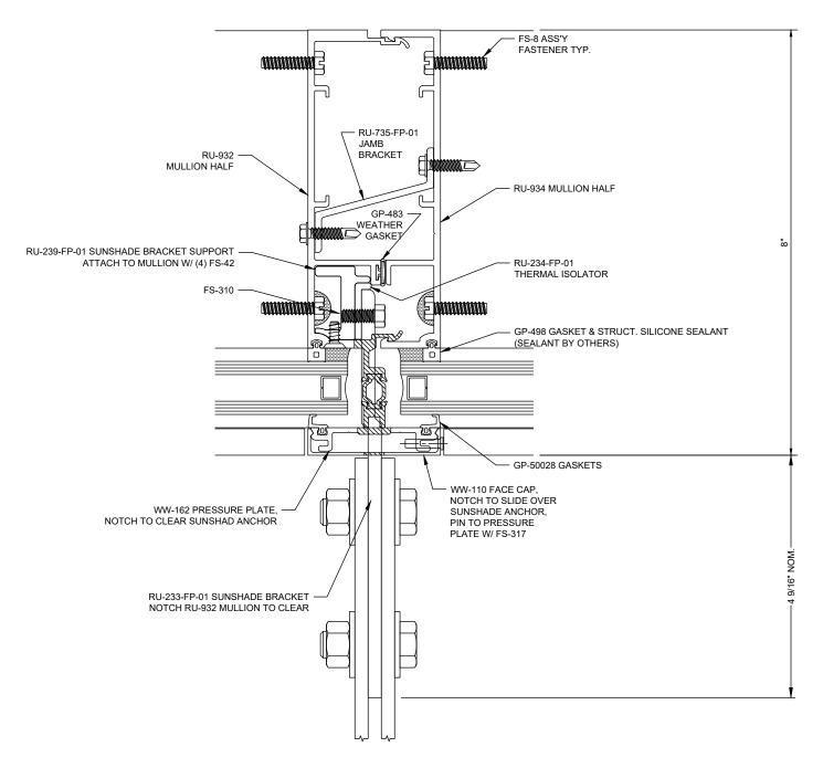
Reliance™ Unit Wall - Captured SSG Sunshade Anchoring at Intermediate Vertical - V1892
