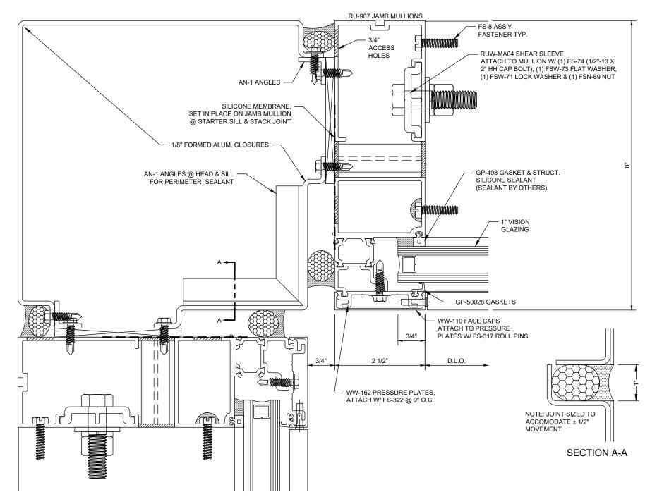
Reliance™ Unit Wall - Captured SSG 90° Inside Corner @ Stack Joint - V1876
