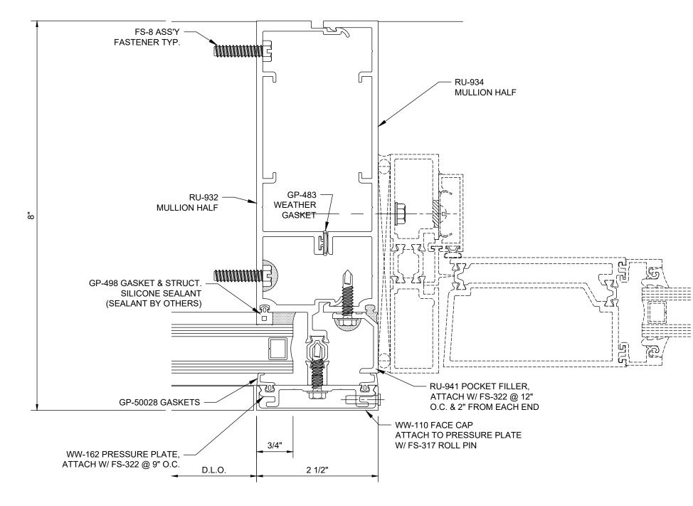
Reliance™ Unit Wall - Captured SSG Vertical @ Thermal Door Jamb - V1882
