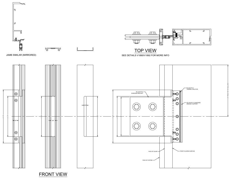
Reliance™ Unit Wall - Captured SSG Sunshade Anchoring at Jamb & Intermediate Verticals - H1890
