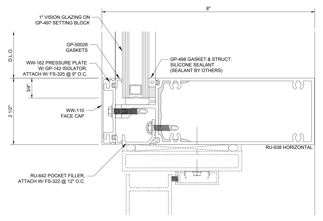
Reliance™ Unit Wall - Captured SSG Horizontal @ Door Header for Overhead Surface Closer - H1880
