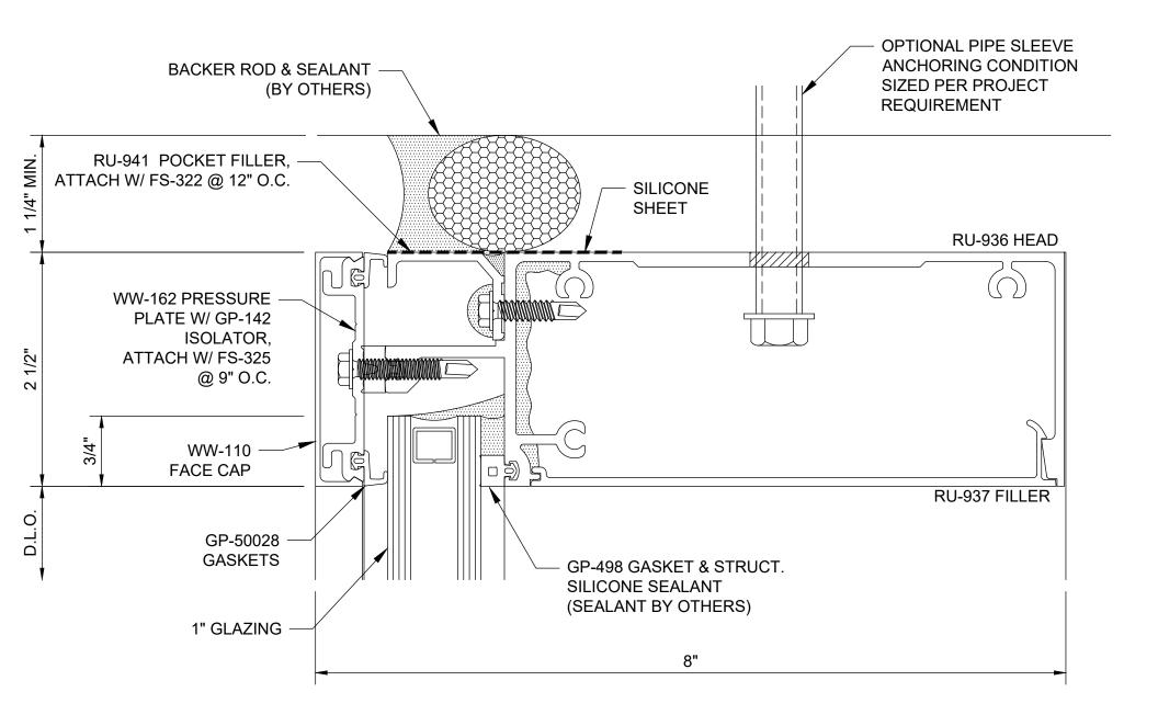
Reliance™ Unit Wall - Captured SSG Head Horizontal - Multi-Span - H1853
