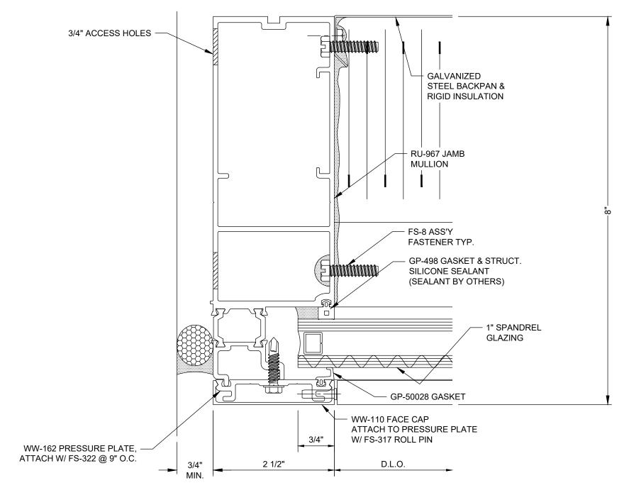
Reliance™ Unit Wall - Captured SSG Jamb Vertical @ Spandrel - V1866
