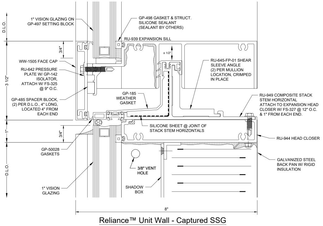
Stack Joint - Vision over Shadow Box w/ Shear Sleeve Angle - H1866
