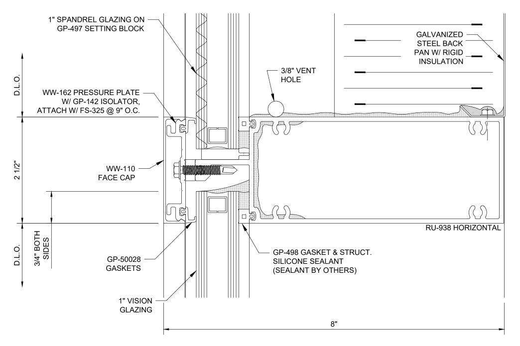
Reliance™ Unit Wall - Captured SSG Intermediate Horizontal @ Spandrel over Vision - H1862
