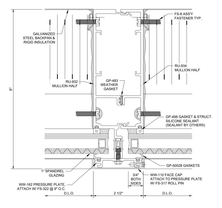
Reliance™ Unit Wall - Captured SSG Intermediate Vertical @ Spandrel - V1861
