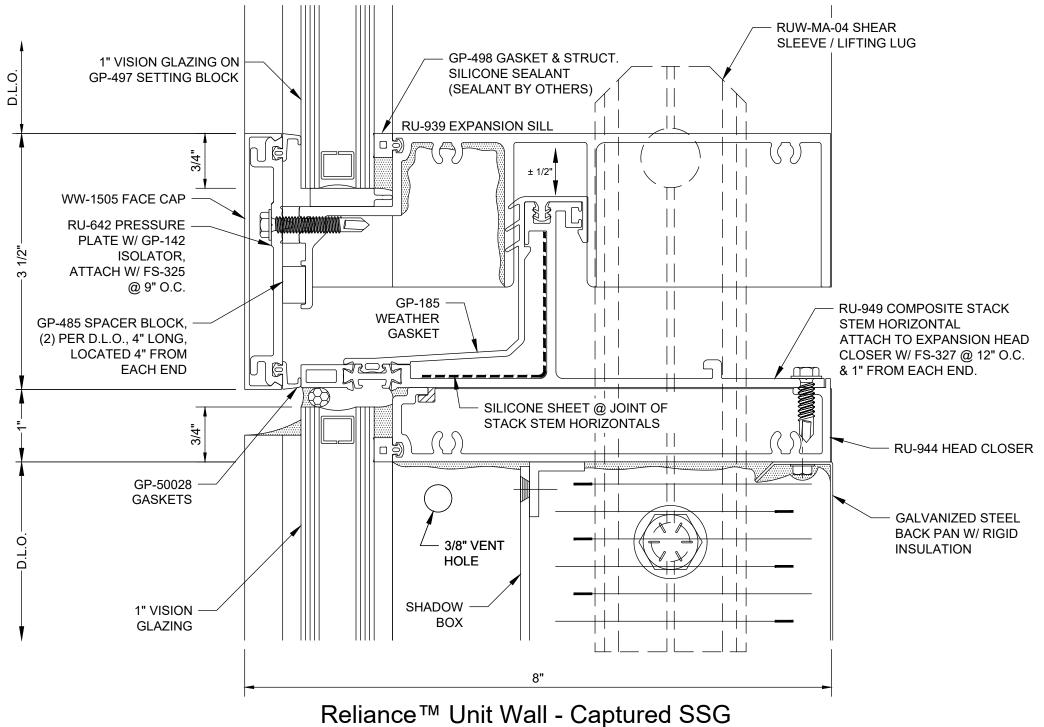
Stack Joint - Vision over Shadow Box w/ Shear Sleeve/Lifting Lug - H1865
