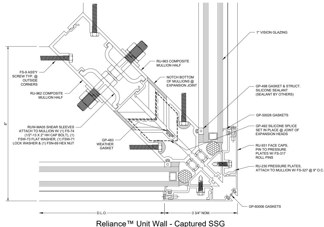
Reliance™ Unit Wall - Captured SSG 90° Outside Corner @ Stack Joint - V1871
