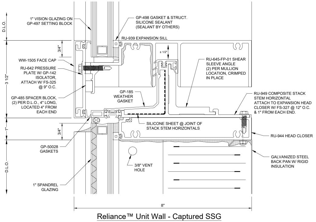
Stack Joint - Vision over Spandrel w/ Shear Sleeve Angle - H1861
