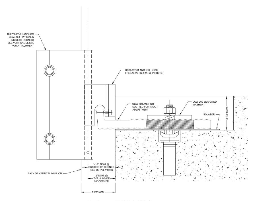
Reliance™ Unit Wall Wind Load Anchor @ Floor Slab - H1802
