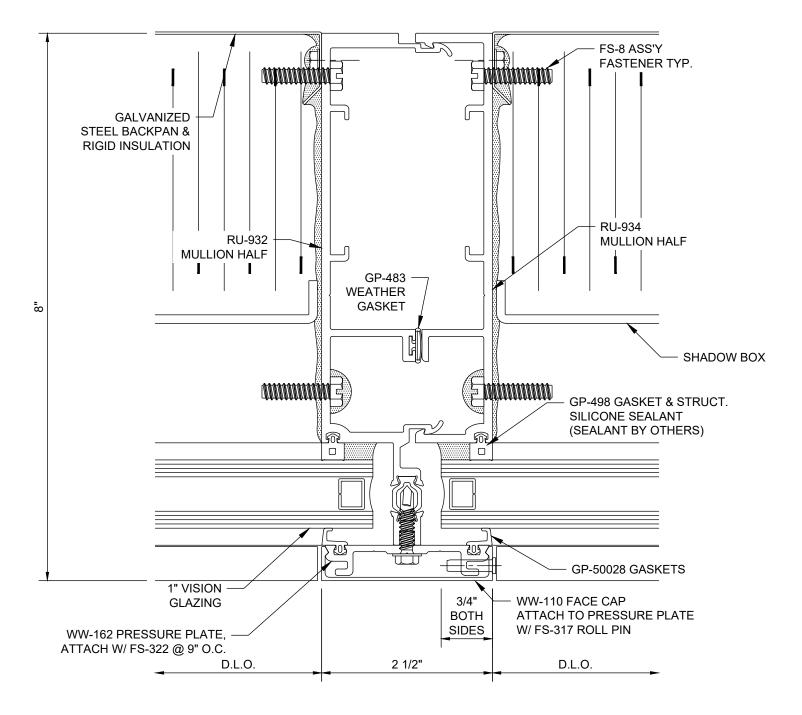
Reliance™ Unit Wall - Captured SSG Intermediate Vertical @ Shadow Box - V1862
