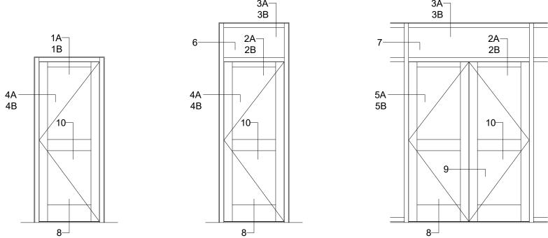
9/16" MONOLITHIC LAMINATED GLAZING IN DOOR, 9/16" MONOLITHIC LAMINATED GLAZING IN FRAME NOTE: DRY GLAZED TRANSOM NOT SUPPORTED
