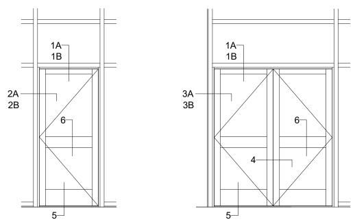
9/16" MONOLITHIC LAMINATED GLAZING IN DOOR, 1-5/16" INSULATING LAMINATED GLAZING IN FRAME
