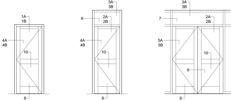
9/16" MONOLITHIC LAMINATED GLAZING IN DOOR, 1-5/16" INSULATING LAMINATED GLAZING IN FRAME NOTE: DRY GLAZED TRANSOM NOT SUPPORTED
