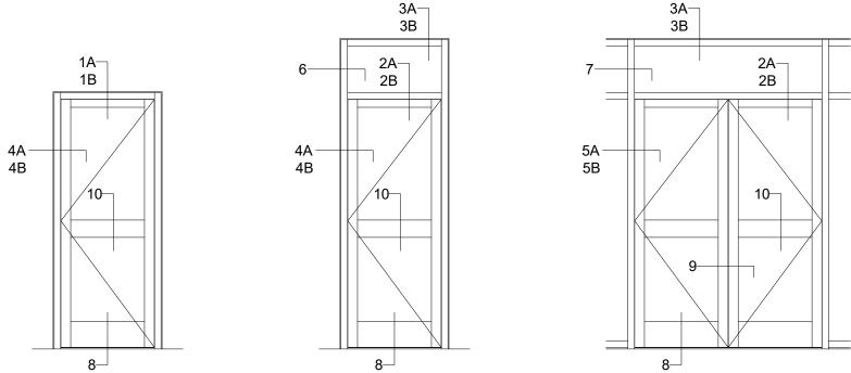
9/16" MONOLITHIC LAMINATED GLAZING IN DOOR, 9/16" MONOLITHIC LAMINATED GLAZING IN FRAME NOTE: DRY GLAZED TRANSOM NOT SUPPORTED
