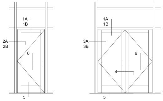
9/16" MONOLITHIC LAMINATED GLAZING IN DOOR, 1-5/16" INSULATING LAMINATED GLAZING IN FRAME
