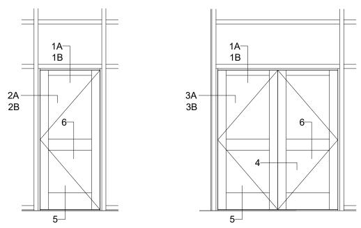
9/16" MONOLITHIC LAMINATED GLAZING IN DOOR, 9/16" MONOLITHIC LAMINATED GLAZING IN FRAME
