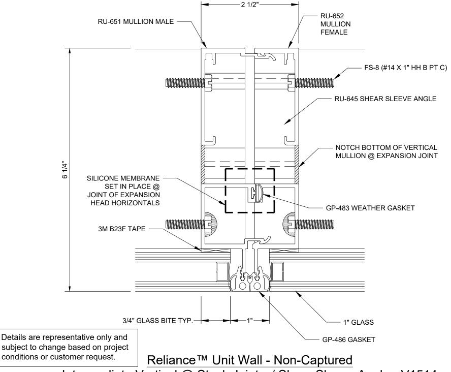
Intermediate Vertical @ Stack Joint w/ Shear Sleeve Angle - V1514
