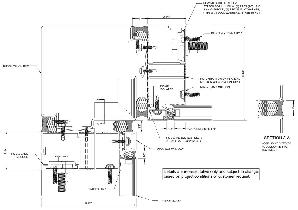
Reliance™ Unit Wall - Non-Captured 90° Inside Corner @ Stack Joint - V1526
