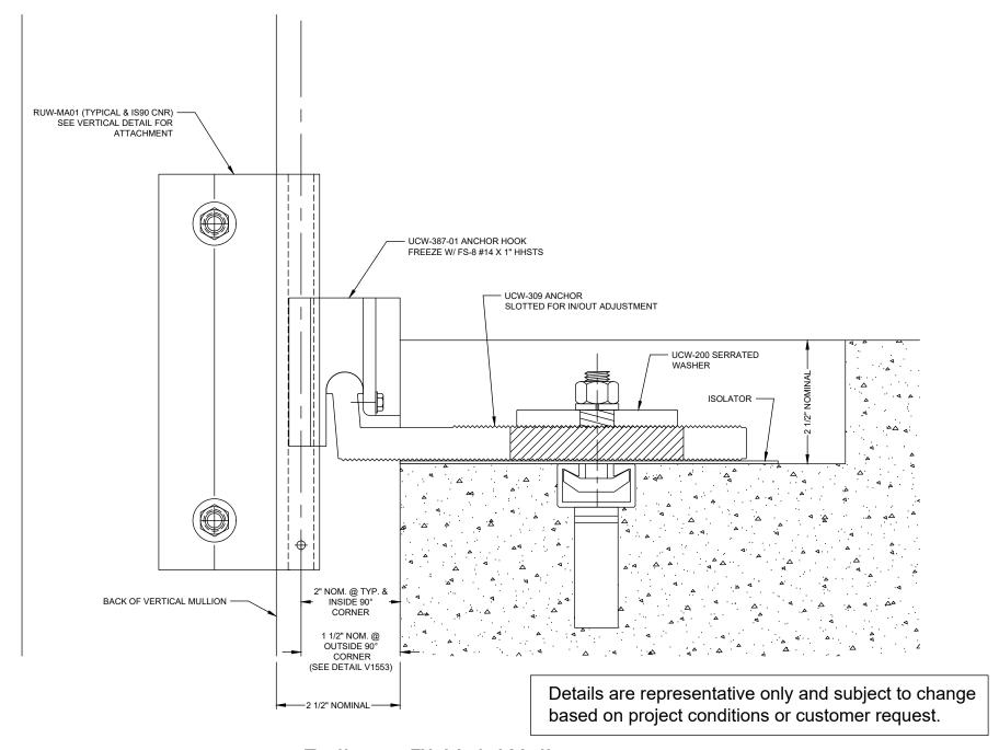
Reliance™ Unit Wall Windload Anchor @ Floor Slab - H1502
