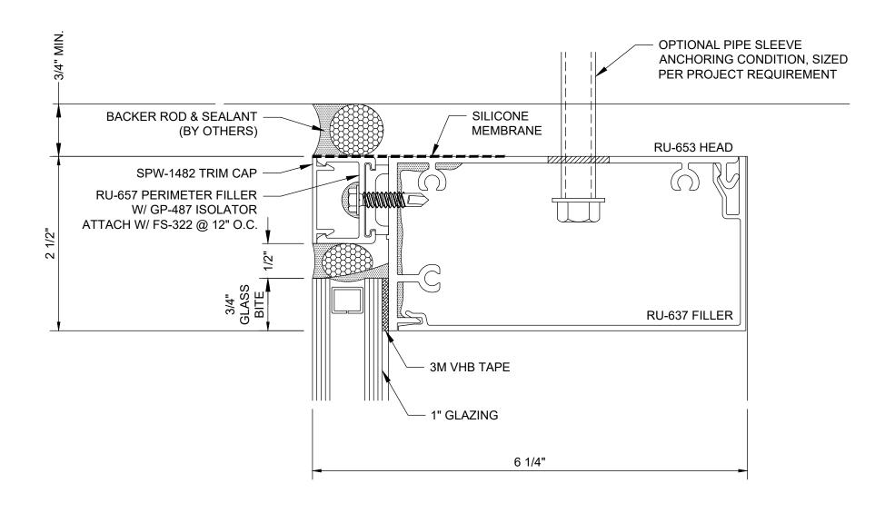
Reliance™ Unit Wall - Non-Captured Head Horizontal - Single Span - H1504
