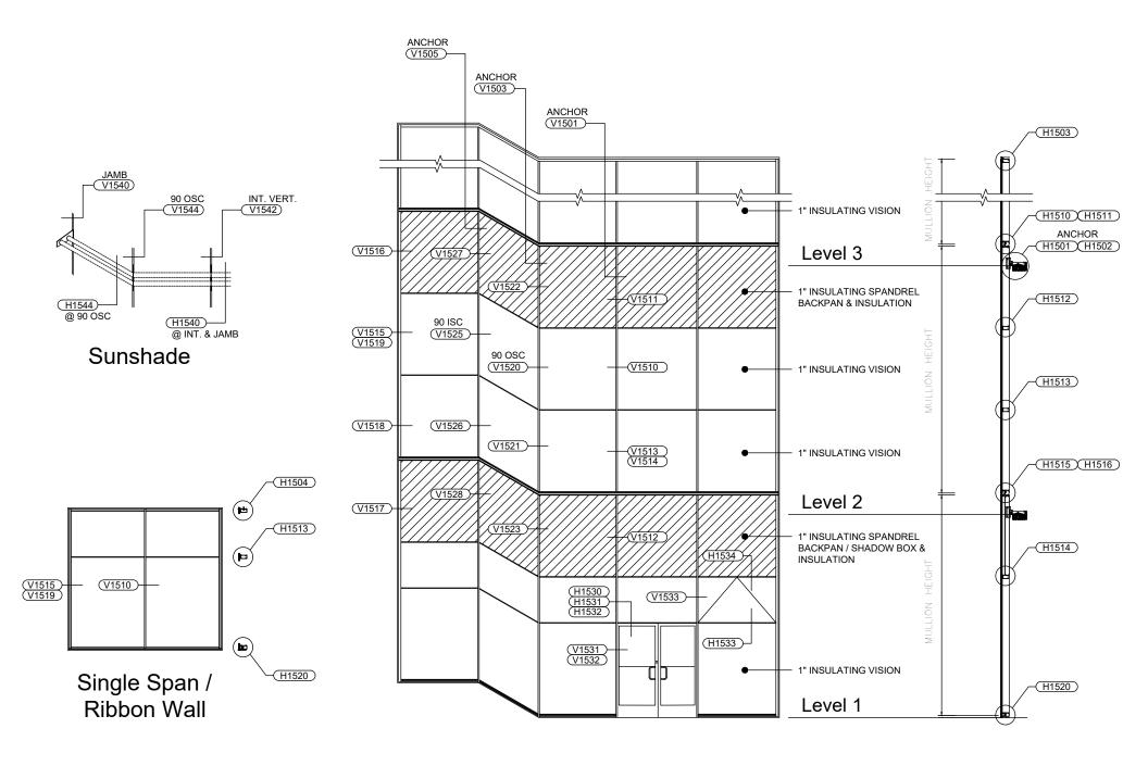
Reliance™ Unit Wall - Non-Captured - Structural Tape Glazed 2-1/2" x 6-1/4" w/ 1" Glazing - Elevation
