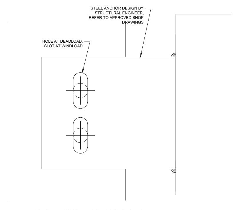
Reliance™ StormMax® High Performance Steel Anchoring at Face of Slab - M9644
