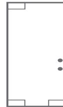
F Style Patch fittings at top and bottom and a lock patch at the leading edge of the door
