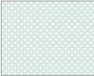
Dots —40% coverage; 1/8" dots staggered on 1/4" centers
