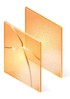
eat-treated glass offers increased resistance to impact, wind loads and thermal stress breakage. Annealed glass is heated to approximately 1,150°F (621°C) and rapidly air-cooled to become heat-strengthened or fully tempered.
